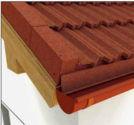
Adjust the Box Barges in a straight line and fix them using nails or fasteners. Note that the fasteners need to be near the bottom edge of the Box Barge to ensure that the bottom edge is firmly positioned against the barge board.
